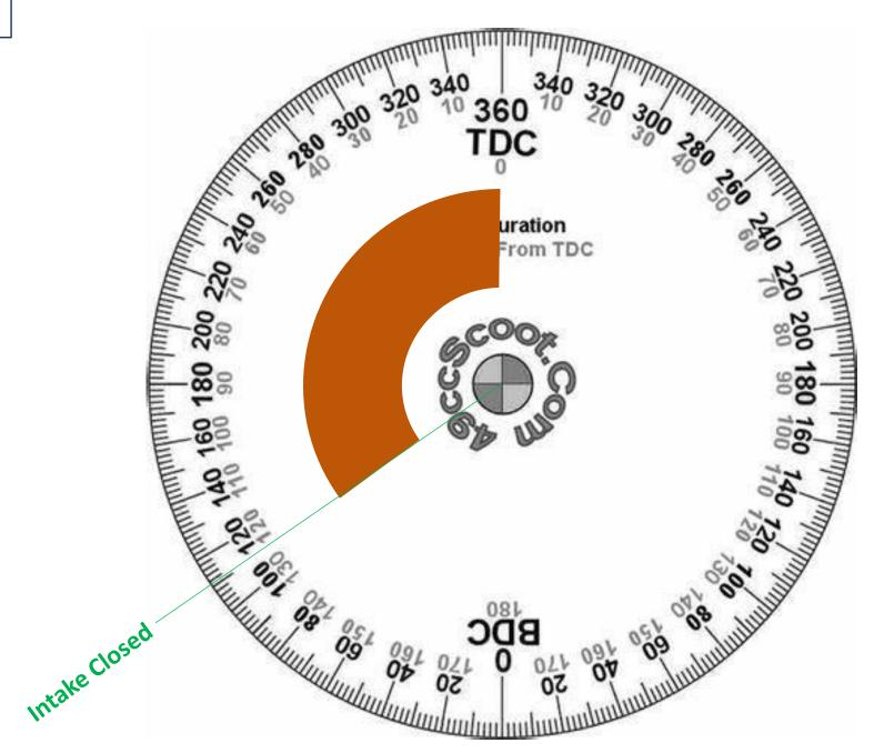
Intake Duration: °290 Compression: 125° Power Stroke: 125° Exhaust Duration: 260°
