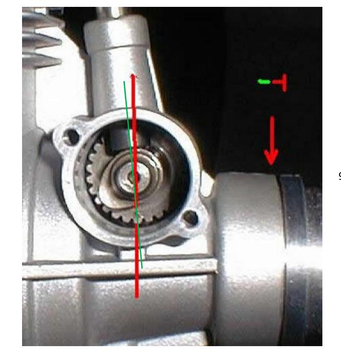
Proper alignment (green) is with the pushrod tubes, not 90° to the crankcase web (TF)
