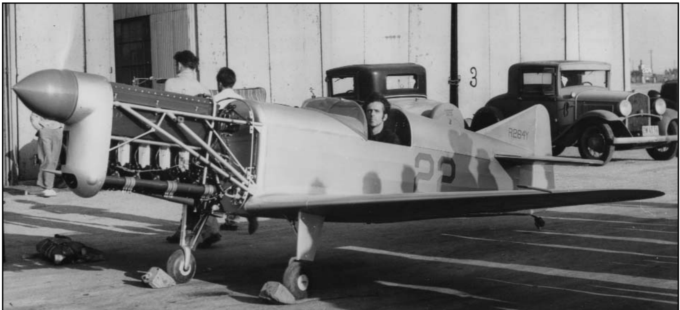
Running up the uncowed Menasco in the Keith Rider R-5 (David Ostrowski)
