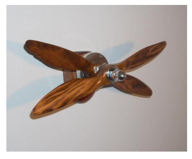
Weight of props and gearbox assembly is 6 ounces (231 gr) including new chrome acorn nut and stainless steel face washer. Wood mounting and hardware estimated to weigh 2 ounces (5 gr). Sun gear is 24 teeth, first planet gear is 8 teeth, second planet gear is 16 teeth, brass ring gear is 48 teeth.
