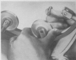
Figure 91—Installing Roller Assembly Into Piston Forks
