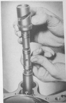
Figure 133—Installing Distributor Valve Assembly and Cam Into Hub
