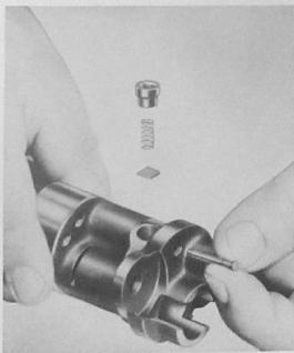
Figure 82—Assembling Low Pressure Check Valve—Composite View
