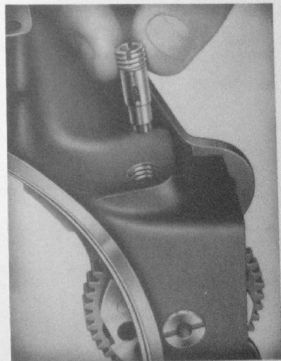
Figure 192—Inserting Ratchet Wheel Lock Assembly
