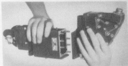
Figure 215—Installing Servo Motor Onto Governor
