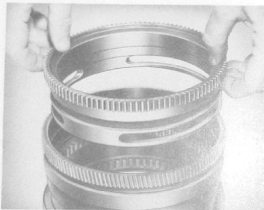
Figure 96—Placing Governor Drive Gear Inside Eccentric
