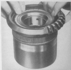
Figure 105—Installing End Plate Gasket
