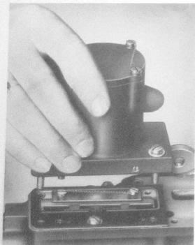
Figure 211—Assembling Pitch Limit Solenoid to Control Support
