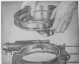
Figure 209—Assembling Translating Control Onto Control Support
