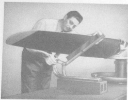
Figure 120—Setting Blade Angles
