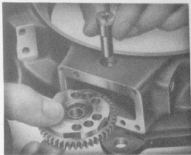
Figure 191—Assembling Auxiliary Motor Ratchet Wheel—Composite View
