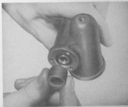
Figure 140—Inserting End Cover Bushing
