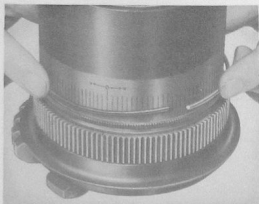
Figure 109—Installing Micro-Adjustment Ring Snap Ring
