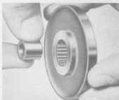
Figure 89— Inserting Inner Race Into Roller
