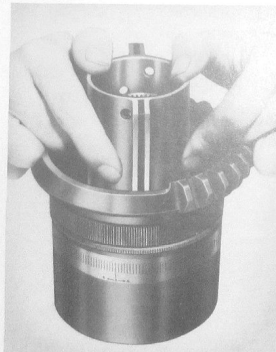
Figure 102—Installing Barrel Vane Into Blade Vane
