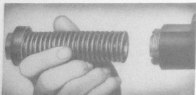
Figure 205—Installing Servo Springs Into Support
