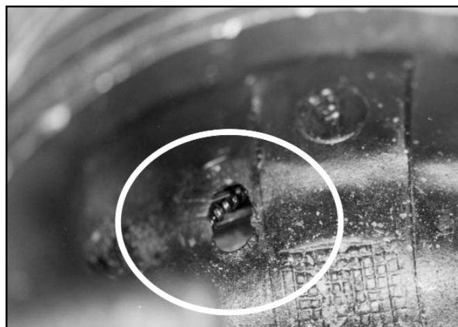
A view of the underside of the same piston shows oil hole enlarged by flames (circle). This allows significant blow-by, which pressurizes the crankcase and rapidly depletes the oil supply, resulting in further engine damage. (Les Waters)
