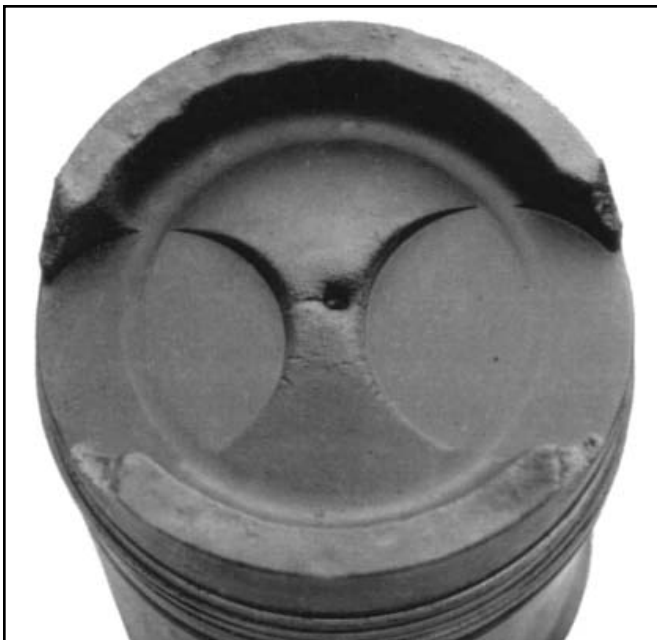
A 10" dual-fuel piston from an engine used to power large electric generators. The piston has been subjected to pre-ignition. Note that, unlike the detonation example, the thermal damage is evenly spread over the piston crown. The piston is made of nodular cast iron, which melts at more than 2,000°F. It must have been subjected to an enormous heat load! The small depression at the center accommodates an eye-bolt used to remove the piston for service. (Les Waters)
