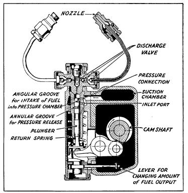
Fig. 41.—Junkers fuel injection pump and its two injectors.
