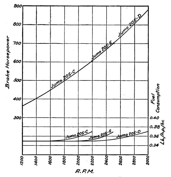
Fig. 46.—Power and fuel consumption curves.
