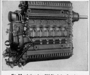
Fig. 35.-Junkers Jumo 205 Diesel aircraft engine.
