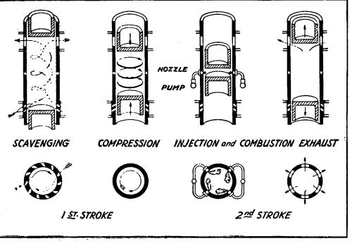
Fig. 36.—Functioning of piston-controlled ports.
