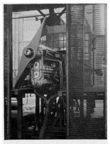
Fig. 45.—Junkers Jumo 205 Diesel on test stand.
