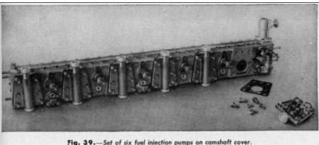
Fig. 39.-Set of six fuel injection pumps on camshaft cover.
