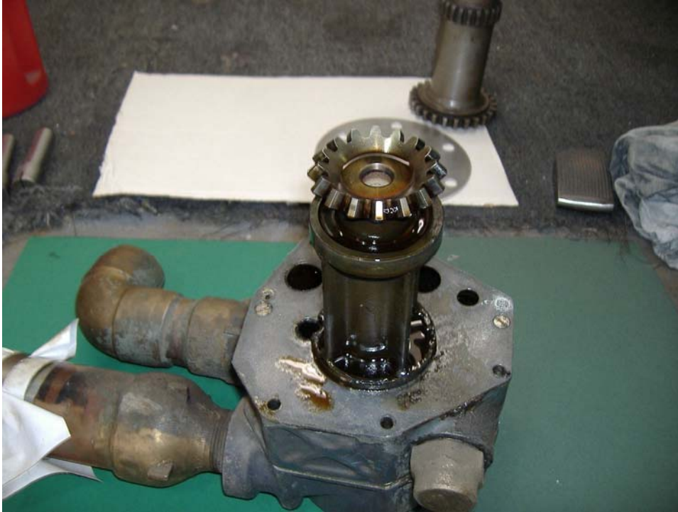
Figure 8 Oil Pump, with Marine Type Brass Fittings as used on V-3420-A8 engines.
