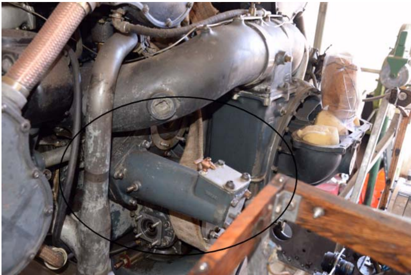
Figure 6 The Throttle Governor support also provides a pad for a Vacuum Pump
