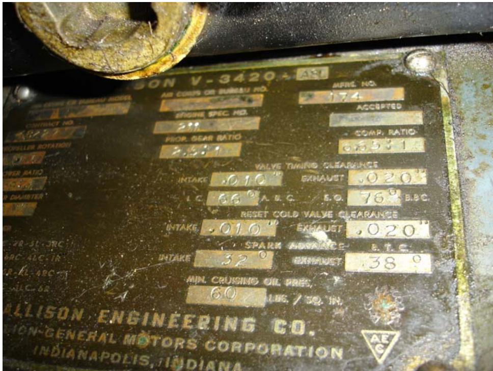
Figure 3 Data Plate on Kermit Weeks V-3420-A8L #174. Note, the Intake Valve clearance of 0.010” was changed on all Air Corps V-1710s to 0.015” in May 1941 to eliminate backfiring. It is curious that the change was not stamped on #174’s data plate when the engine went through overhaul for Gar Wood in Spring 1942.
