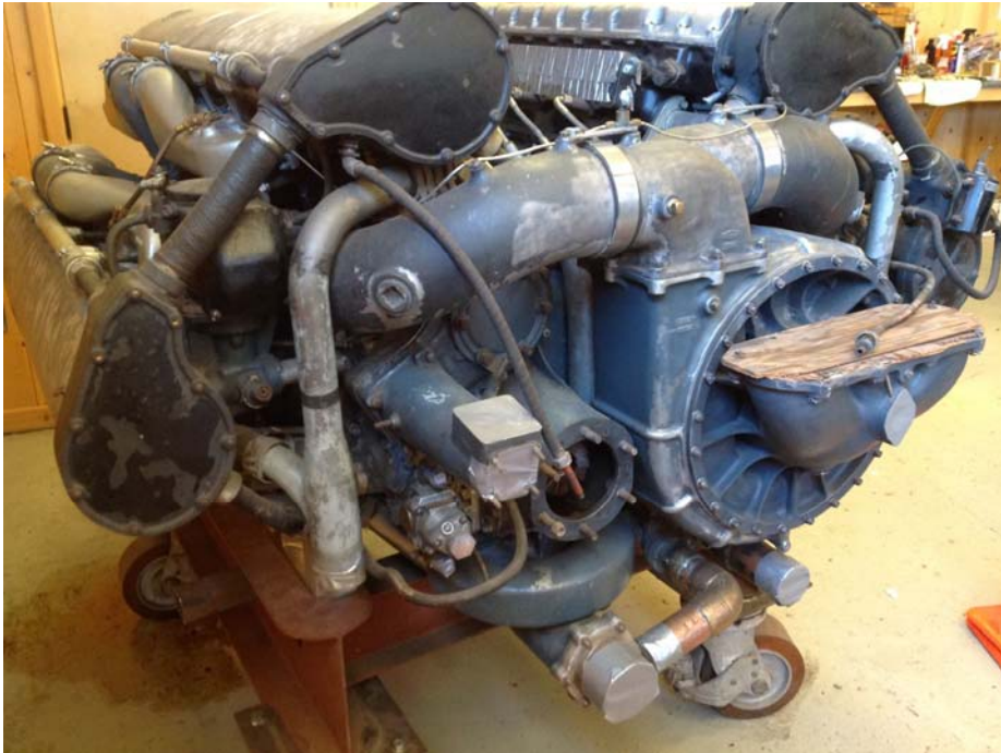
Figure 14 Aft end of V-3420-A8R #173 showing the coolant return pipes (curved-vertical) exiting from the aft end of each cylinder bank. Note also the Throttle Governor pedestal and Vacuum Pump mount as well as the brass pipe fittings on the oil pump.
