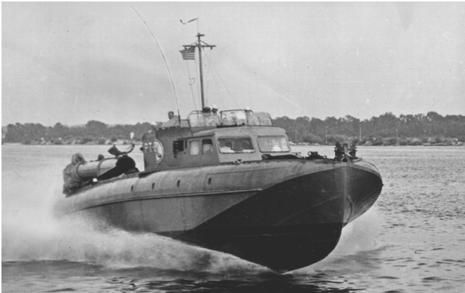
Figure 1 The Navy's Allison V-3420-A8 powered PT-8 underway during testing.
