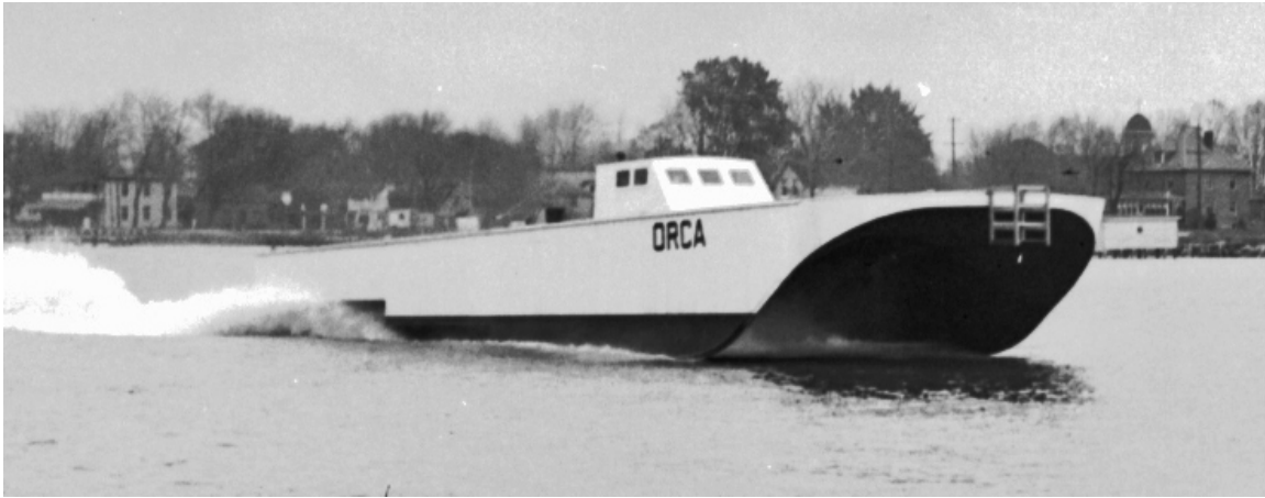
Figure 17 Gar Woods ORCA featured a stepped hull that was essentially “split” in half making it into a catamaran. Its development was lengthy, troubled by details regarding hull shaping.
