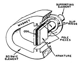
Figure 3.4 Torsiograph Electrical Components (Draper <sup>7</sup>)
