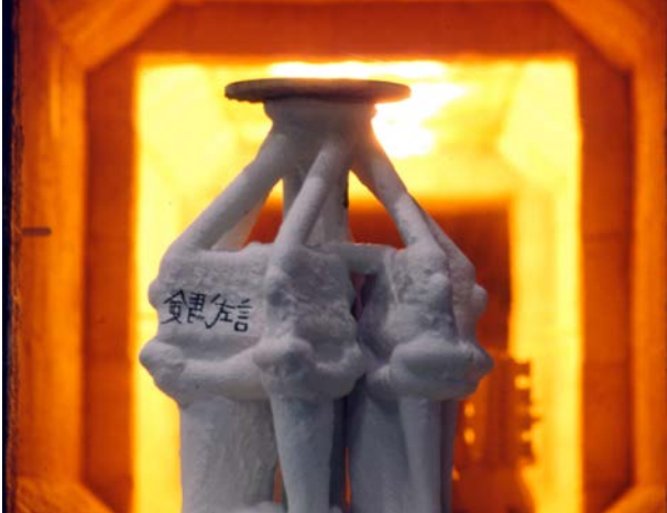
A ceramic mold created by repeatedly dipping wax molds of turbine blades into a ceramic slurry gets ready to go into the vacuum furnace at Howmet's Terai, Japan foundry. There it will be filled with molten superalloy to form directionally solidified turbine blades. (Photo courtesy of Howmet Corp.)
